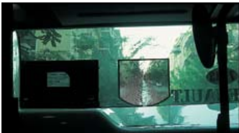
Wide-angled lens in rear window providing view of area behind bus (Athens, 2005, ordinary city bus).
