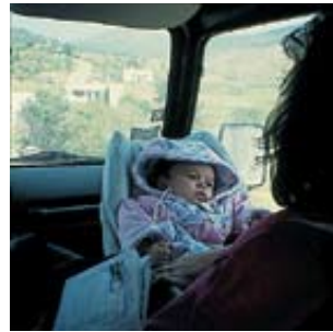
Proper installation of seat with child's back to the windscreen – but all wrong in every other respect! The child's seat is placed in the front passenger position to the right of the mother (where it is doubtful if the car seatbelt will be an adequate restraint), and the mother, with no seatbelt, would be thrown onto the child in the event of a collision. Good intentions aren't enough! (Evia, 1997).
