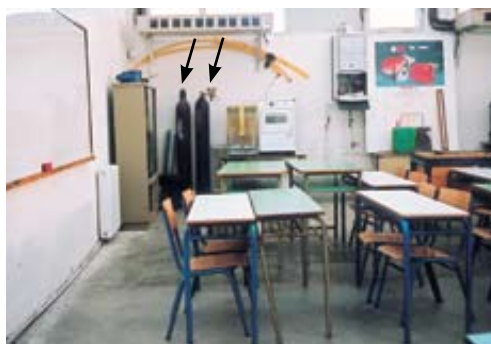
Note the unsupported gas cylinders, as well as other safety problems (Thessaloniki, 2005).
