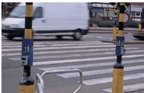
At this pedestrian crossing in the Netherlands an audible signal tells the blind when it is safe to cross. Similar devices installed at some crossings in Greece have been damaged or removed! Even where these devices exist in Greece, it is not always safe to rely on them – too many vehicles ignore the lights!
